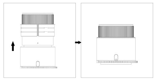
3. Align the lens index mark with the hole on the aluminum ring, insert the aluminum ring onto the plastic c-ring until it reaches the flange of the plastic c-ring.
