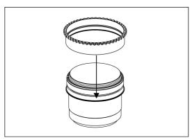
Insert the gear of SE30-F on the plastic c-ring until it reaches the flange of the plastic c-ring.
