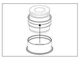
Insert the gear of P1442-Z on the plastic c-ring until it reaches the flange of the plastic c-ring.
