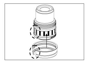
1. Insert the plastic c-ring as shown and place it over the lens rubber zoom ring.
