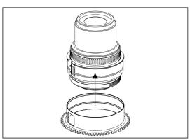
2. Insert the gear of O918-Z on the plastic c-ring until it reaches the flange of the plastic c-ring.
