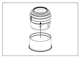
2. Insert the gear of P45-F on the plastic c-ring until it reaches the flange of the plastic c-ring.
