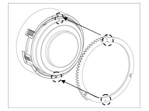
3. Align the pins on the cover with the holes in the gear ring as indicated in the diagram.
