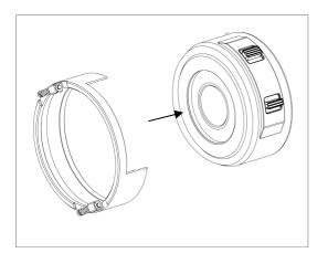
1. Align the base unit of the zoom gear with the lens as indicated in the diagram. Then lightly push the base unit towards the lens until it cannot go any further.
