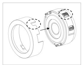
2. Align the zoom lever on the lens with the opening of zoom gear cover as indicated in the diagram. Then lightly push the cover towards the lens until it cannot go any further. Make sure the two springs on the base unit sit inside the groove in the cover (not shown).
