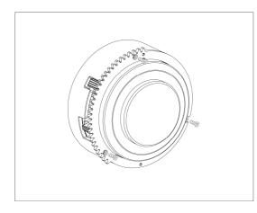
4. Tighten the three screws with a Philips-head screwdriver.
