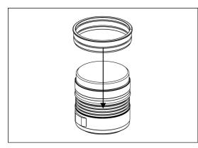
2. Insert the plastic c-ring as shown and place it onto the rubber ring recess of the lens.
