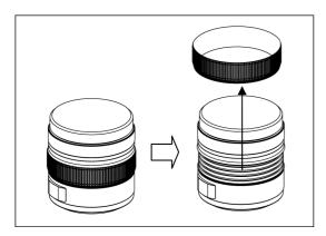
1. Remove the rubber ring from the lens carefully.
