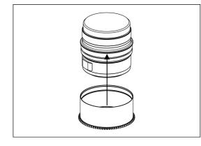
3. Insert the gear of P1235-Z on the plastic c-ring until it reaches the flange of the plastic c-ring.
