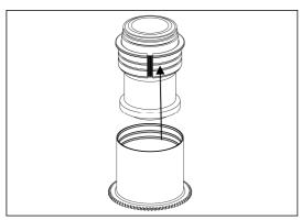
2. Insert the gear of O6o-F on the plastic c-ring until it reaches the flange of the plastic c-ring.
