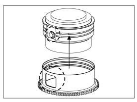
2. Align the "opening" of the gear with the button on the lens barrel. Insert the gear of N1030-Z on the plastic c-ring until it reaches the flange of the plastic c-ring.
