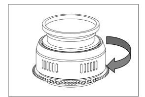
4. Tighten the zoom gear by turning the outer ring clockwise while holding the toothed part firmly, until it cannot go in any further.
