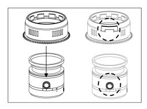
3. Align the "opening" of the gear with the button on the lens barrel. Insert the gear of N6.713-Z as shown and place it over the lens zoom ring.
