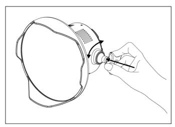
2. Engage the gear by pushing in the knob, then turn the knob both ways to check if the lens focuses.
