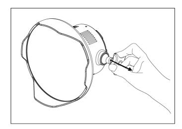
Make sure the control knob is at its most outwards position before mounting/ unmounting the port. The knob should be left at this position until it is made sure that the lens and focus gear is properly installed.
