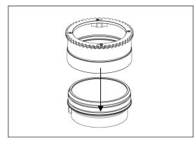
2. Insert the gear of SE1650-Z on the plastic c-ring until it reaches the flange of the plastic c-ring.
