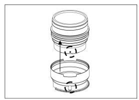
3. Align the lens index mark with the opening on the gear of SE1018-Z, insert the gear of SE1018-Z on the plastic c-ring until it reaches the flange of the plastic c-ring.
