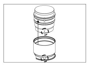
3. Align the lens index mark with the opening on the gear of SE1670-Z, insert the gear of SE1670-Z on the plastic c-ring until it reaches the flange of the plastic c-ring.
