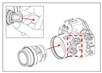
Make sure the two knobs are at its most outwards position before mounting/un-mounting the lens. The knobs should be left at this position until it is made sure that the lens and gear is properly installed.
