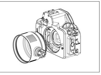
Align the port mounting indices of B and the housing. Gently push B into the port opening of the housing, until it cannot go in any further.
