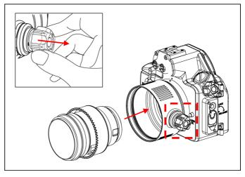
Make sure the zoom knob is at its most outwards position before mounting/ un-mounting the lens. The knob should be left at this position until it is made sure that the lens and zoom gear is properly installed.
