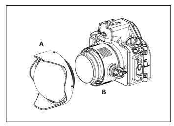
Remove the O-ring from A, inspect for any damage and lightly coat it with the provided lubricant. Clean the O-ring groove before placing it back.
