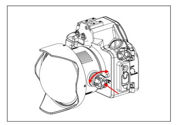
Attach A on B by holding the housing firmly and turning A clockwise until it cannot go in any further.
