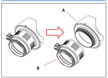
Detach A from the port by turning it anti-clockwise while holding B firmly.
