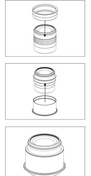
1. Insert the plastic c-ring as shown and place it over the lens zoom ring.
