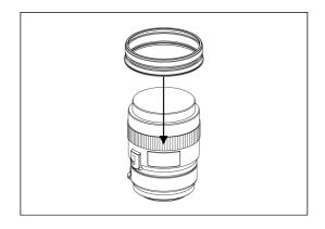
1. Insert the plastic c-ring as shown and place it over the lens rubber focus ring.
