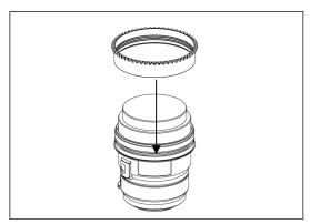
2. Insert the gear of CMEF60-F on the plastic c-ring until it reaches the flange of the plastic c-ring.
