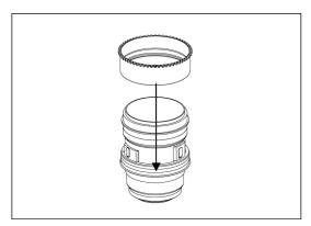
2. Insert the gear of CMEF815-Z on the plastic c-ring until it reaches the flange of the plastic c-ring.
