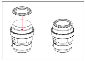
Mount the alignment ring onto the lens by screwing it into the thread on the front of the lens.
