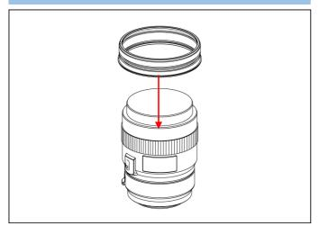
Insert the plastic c-ring as shown and place it over the lens rubber focus ring.
