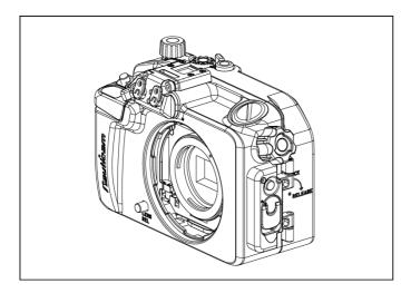
Install the camera body only into the housing.
