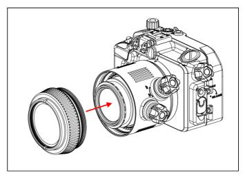
Remove the O-ring from A, inspect for any damage and lightly coat it with the provided lubricant. Clean the O-ring groove before placing it back.
