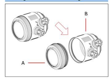
Detach A from the port by turning it anti-clockwise while holding B firmly.
