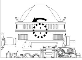
Turn the port anti-clockwise until the white dot on the adaptor aligns with the white dot on the port.
