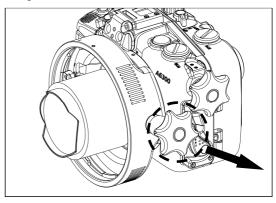
Mount the lens (with gear attached) on the camera.
