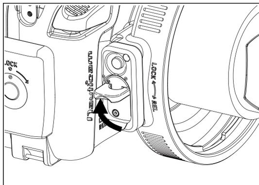
Lift the Port lock/ release latch on the other side of the adaptor.
