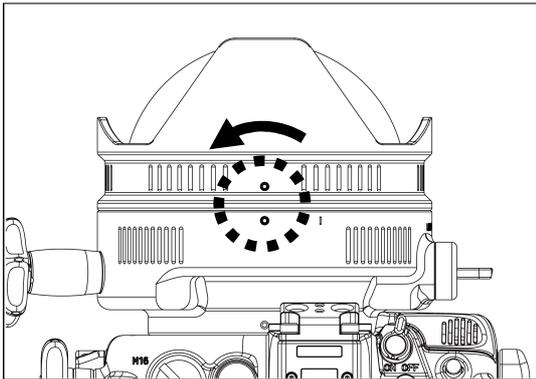
Turn the port anti-clockwise until the white dot on the adaptor aligns with the white dot on the port.
