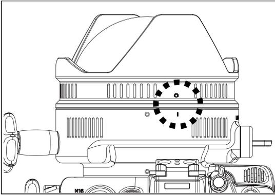
Align the "I" mark on the adaptor with the WHITE dot on the port. Gently push the port towards the adaptor until it cannot go in any further.
