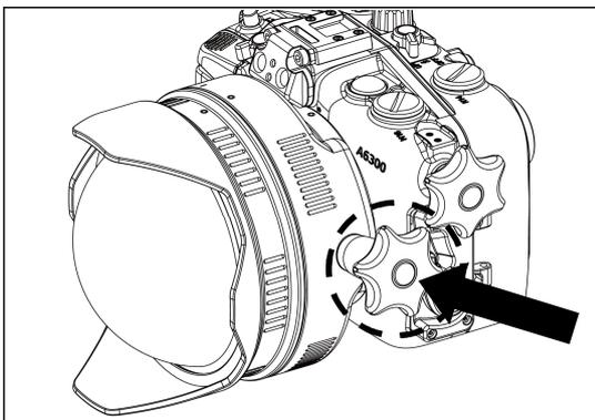
For port adaptor with knob, engage the gear on the lens by pushing the knob inwards, then turn the knob both ways to check if the lens is functioning
