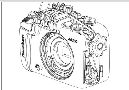
Install the camera body only into the housing and attach the optical fiber cables to the housing.
