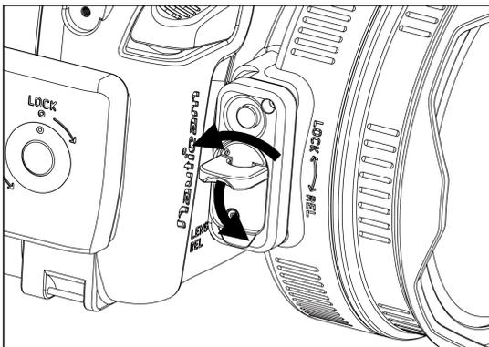
To lock the port in place, turn the port lock/release latch anti-clockwise to the original position and then flip it down.
