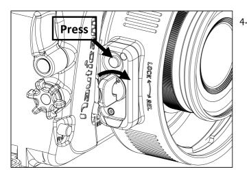
Press and hold the port release safety button, turn the port lock/release latch clockwise until it stops.
