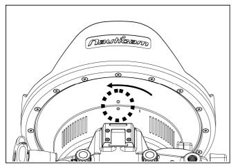
6. Turn the port anti-clockwise until the white dot on the adaptor aligns with the white dot on the port.
