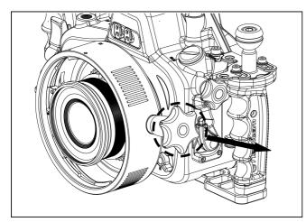
2. Mount the lens (with gear attached) on the camera.
