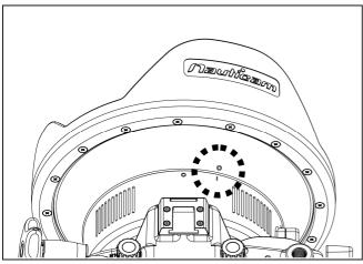
5. Align the "I" mark on the adaptor with the WHITE dot on the port. Gently push the port towards the adaptor until it cannot go in any further.
