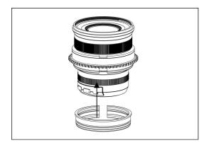
1. Insert the plastic c-ring as shown and place it over the lens aperture ring area.
