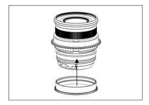
2. Insert the gear of X1024-A on the plastic c-ring until it reaches the flange of the plastic c-ring.
