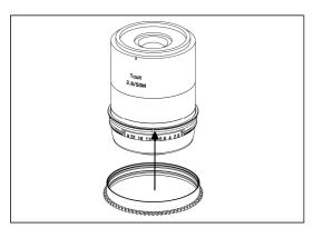
2. Insert the gear of XZ50-A on the plastic c-ring until it reaches the flange of the plastic c-ring.
