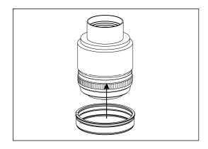
1. Insert the plastic c-ring as shown and place it over the lens aperture ring area.
