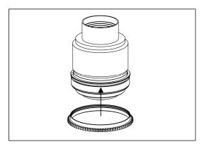
2. Insert the gear of X60-A on the plastic c-ring until it reaches the flange of the plastic c-ring.
