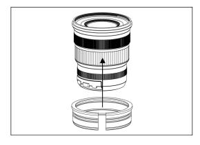
1. Insert the plastic c-ring as shown and place it over the lens zoom ring area.
