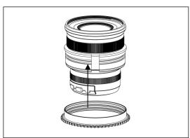
2. Insert the gear of X1024-Z on the plastic c-ring until it reaches the flange of the plastic c-ring.
