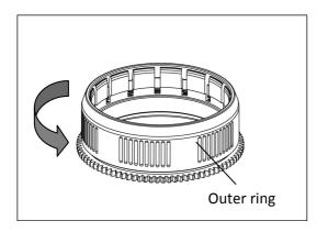
Loosen the zoom gear by turning the outer ring anticlockwise while holding the toothed part firmly, until it can be inserted onto the lens.
