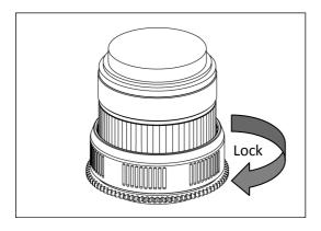
3. Tighten the zoom gear by turning the outer ring clockwise while holding the toothed part firmly, until it cannot go in any further.
