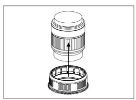
2. Insert the zoom gear as shown and place it over the lens zoom ring until it cannot go in any further.
