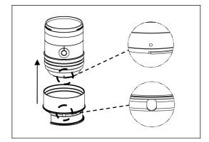
4. Align the lens index mark with the opening on the gear of SEA1635-Z, insert the gear of SEA1635-Z on the plastic c-ring until it reaches the flange of the plastic c-ring.
