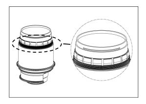
3. Line up the top edge of the focus gear with the lens focus rubber ring. Make sure the focus gear can rotate freely.
