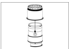
2. Insert the focus gear as shown and place it over the lens focus ring.
