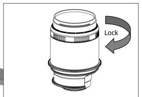
4. Tighten the focus gear by turning the outer ring clockwise while holding the toothed part firmly, until it cannot go in any further.
