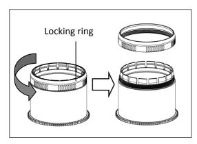
1. Remove the focus gear locking ring by turning the locking ring anti-clockwise while holding the toothed part firmly.
