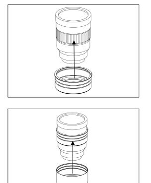
1. Insert the plastic c-ring as shown and place it over the lens zoom ring.
