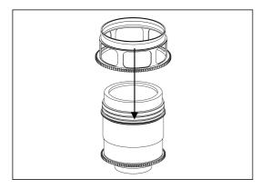
3. Insert the gear of SE1635-F on the plastic c-ring until it reaches the flange of the plastic c-ring.
