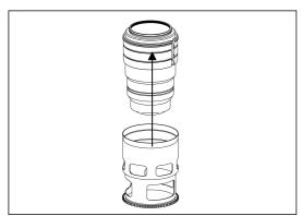
3. Insert the gear of SE90-F on the plastic c-ring until it reaches the flange of the plastic c-ring.
