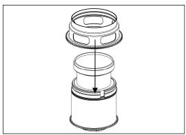
3. Insert the gear of SE2470-F on the plastic c-ring until it reaches the flange of the plastic c-ring.
