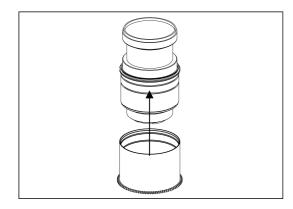
2. Insert the gear of SE2470-Z on the plastic c-ring until it reaches the flange of the plastic c-ring.
