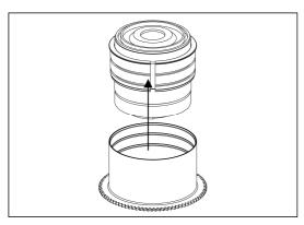
2. Insert the gear of SE28-F on the plastic c-ring until it reaches the flange of the plastic c-ring.
