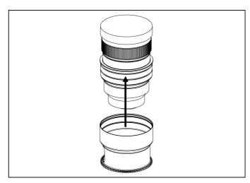
Insert the gear of SFE2470GM-Z on the plastic c-ring until it reaches the flange of the plastic c-ring.
