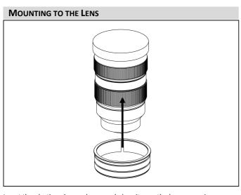
Insert the plastic c-ring as shown and place it over the lens zoom ring.
