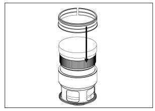
Insert the plastic c-ring as shown and place it over the lens focus ring.
