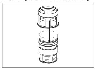
Insert the gear of SFE2470GM-F on the plastic c-ring until it reaches the flange of the plastic c-ring.
