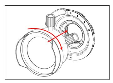
Align the focus knob of the Nikonos lens with the index mark on the adaptor and then gently pushing it into the adaptor until it cannot go in any further.
