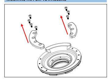
Detach the two section rings from the adaptor by removing the screws.
