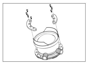
Install the two section rings back onto the adaptor and tighten it with screws.
