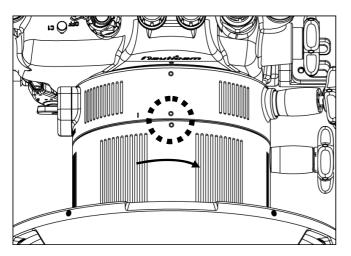
6. Turn the port clockwise until the white dot on the adaptor aligns with the white dot on the port.
