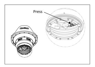
Press the grey button as shown to lock the lock. Ensure that the adaptor is securely locked with the port.
