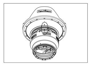
2. Align the "I" mark on the adaptor with the WHITE dot on the port.
