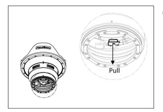
6. To unlock, pull the black locking block towards the port opening and reverse step 4 to 1 to un-mount the port.
