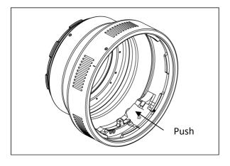
1. Push the black locking block inwards to unlock the adaptor as shown.
