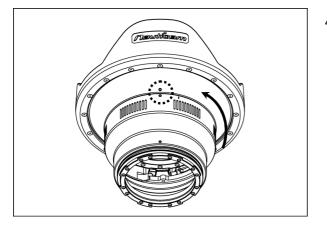
4. Turn the adaptor clockwise until the white dot on the adaptor aligns with the white dot on the port.
