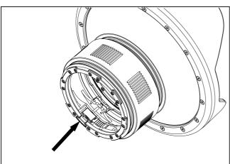
5. Push the locking device inwards. Ensure that the extension ring is securely locked with the port.
