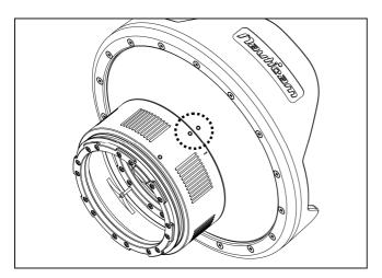
4. Turn the extension ring clockwise until the white dot on the extension ring aligns with the white dot on the port.
