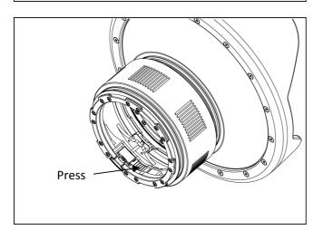
6. To unlock, press the RED bar to release the locking device and reverse the above procedures.
