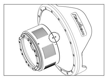
4. Turn the extension ring clockwise until the white dot on the extension ring aligns with the white dot on the port.
