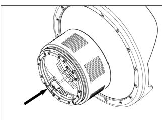
5. Push the locking device inwards. Ensure that the extension ring is securely locked with the port.
