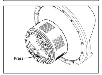
6. To unlock, press the RED bar to release the locking device and reverse the above procedures.
