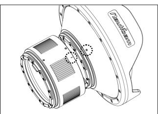
2. Align the "I" mark on the extension ring with the WHITE dot on the port.
