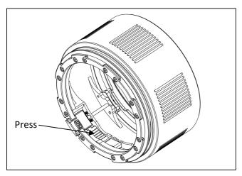
1. Press the RED bar to unlock the locking device of the extension ring.
