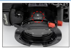
Align the "I" mark on the Port with the "o" mark on the housing, then gently push the port into the port opening of the housing, until it cannot go in any further.
