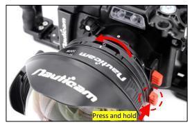
1. Press and hold the RED lens release button and then turn the lens counter clockwise.
