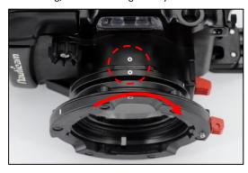
Turn the port clockwise until the "o" mark on the port aligns with the "o" mark on the housing and a "click" sound is heard.
