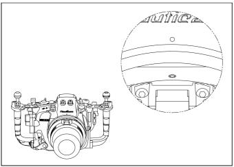
Align the mounting indices of the port and the housing; these appear as white circles on both the port and the housing.
