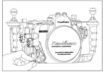
Turn the port locking lever to the release position as shown.
