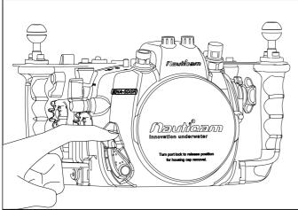
Push the safety button of the port locking lever downwards.
