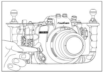
Lock the port into place by turning the port locking lever to the inward position. To ensure that the port is securely mounted, confirm that the green line on the safety button of the port locking lever is visible.
