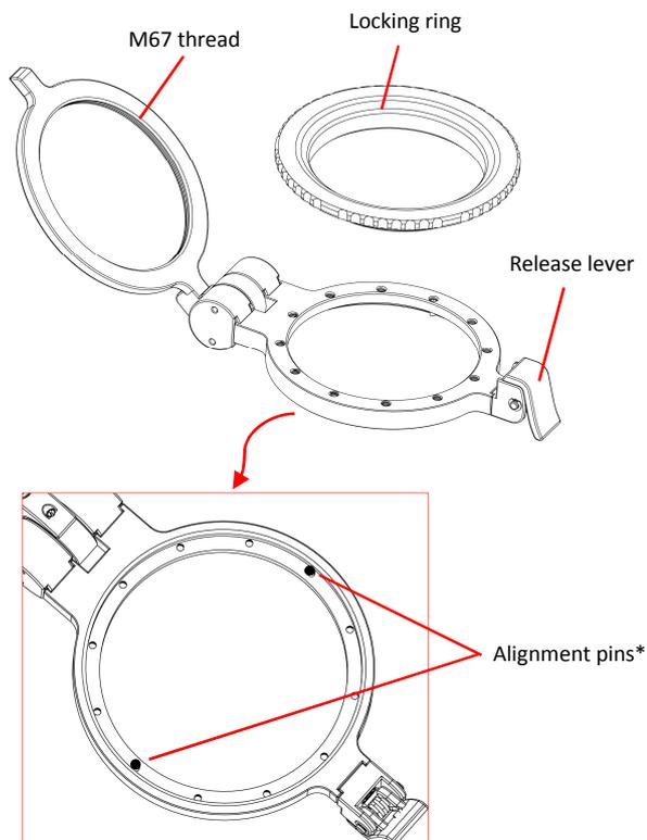
\*There are two alignment pins at the bottom of the holder, by relocating the two screws to the threaded holes around the holder, the position of the holder can be changed.
