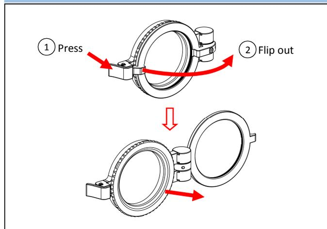
Press the lever and flip the diopter holder to the side then remove the locking ring from the flip diopter holder.
