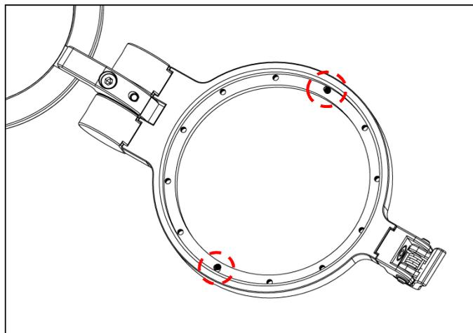
The position of the flip diopter holder can be changed by relocating the two screws in the threaded holes around holder.
