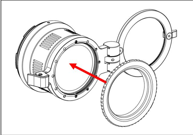
Fasten the holder by screwing the locking ring into the thread on the front of the port.
