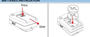
Make sure the On/Off switch is in the OFF position. Remove the battery compartment cover by sliding it outwards.
