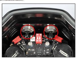
Install the TTL converter and simultaneously insert both LEDs into the optical bulkheads.
