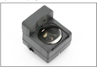
Install the batteries (CR2450 x2pcs) with +ve terminal facing up as shown above. Close the battery compartment cover and then switch the trigger unit on. The indicator will turn green.
